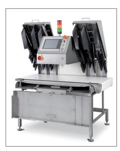
RAYCON D product inspection systems detect all contaminants that due to their density, chemical composition, or mechanical dimensions absorb X-radiation to a lesser or greater degree than the surrounding product. For example, metal, glass, ceramics, and stone contaminants in food. RAYCON D will also detect some plastics (e.g. PVC, rubber) as well as other product defects (e.g. cracks, trapped air). Desired "contaminants" (e.g. aluminium clips on sausage chubs) can be masked out.
