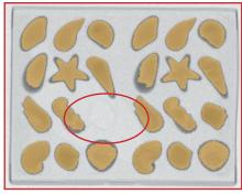
Box with 24 chocolates Integrity checking in sealed non-transparent packaging using a count function, and verifying product position.
